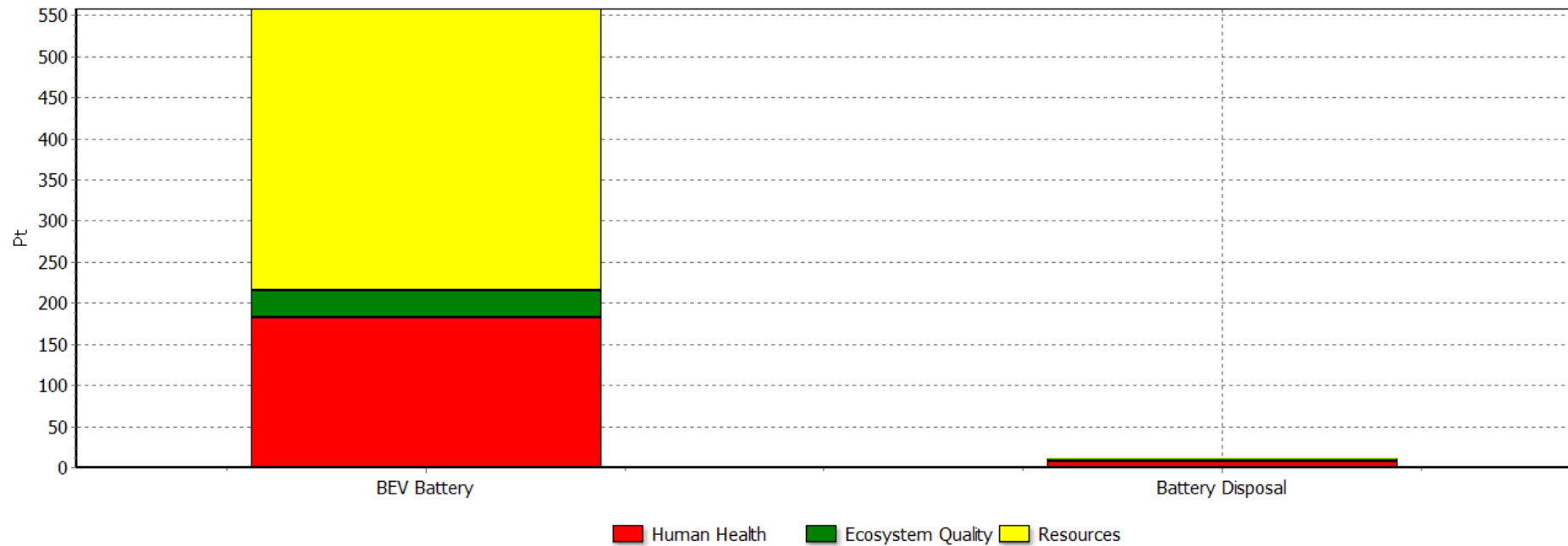
Figure 25 - Contribution of each life stage in the total lifecycle of one battery (Eco-indicator 99) (source: author).
